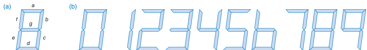
Figure Dec-3 Seven-segment display: (a) segment identification; (b) decimal digits.
