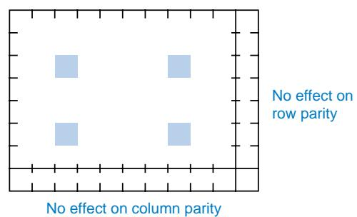
As shown in Figure 2-14(b), the simplest two-dimensional code uses 1-bit even-parity codes for the rows and columns, and has a minimum distance of  $2 \cdot 2$ , or 4. You can easily prove that the minimum distance is 4 by convincing yourself that any pattern of one, two, or three bits in error causes incorrect parity of a row or a column or both. In order to obtain an undetectable error, at least four bits must be changed in a rectangular pattern as in (c).
